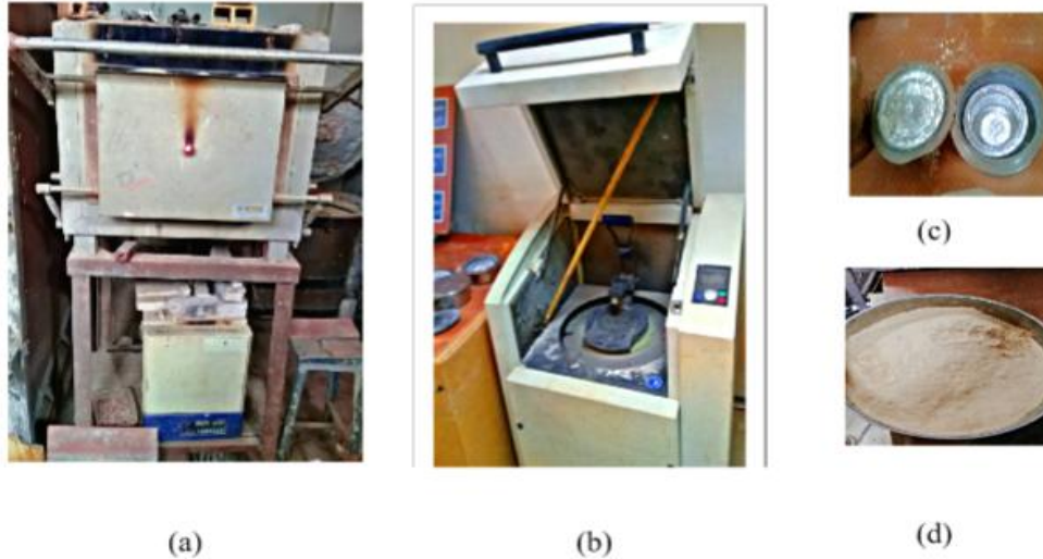
Figure 3. (a) KC Burning Furnace (b) MK Grinding Mill (c) MK Grinding Mold (d) MK Powder
